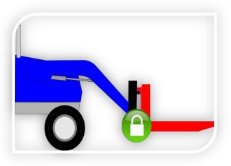
engage the latches on the tractor harness to lock your Skid Steer implement in place.
