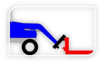
With your tractor, tip the connection harness toward the ground (As if you were emptying a bucket). Lower the loader and bring the tractor harness against your Skid Steer implement.
